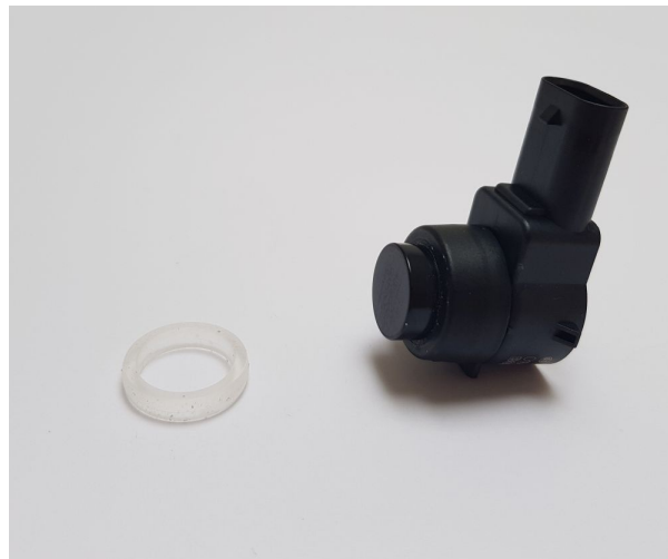
Fig. 5: Ultrasonic sensor Bosch USS4 (X200)
